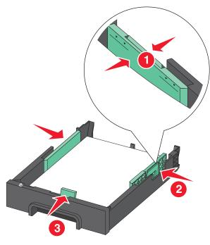
**Note:** Make sure the paper is below the maximum fill line located on the edge of the paper tray. Overloading the tray can cause paper jams.
